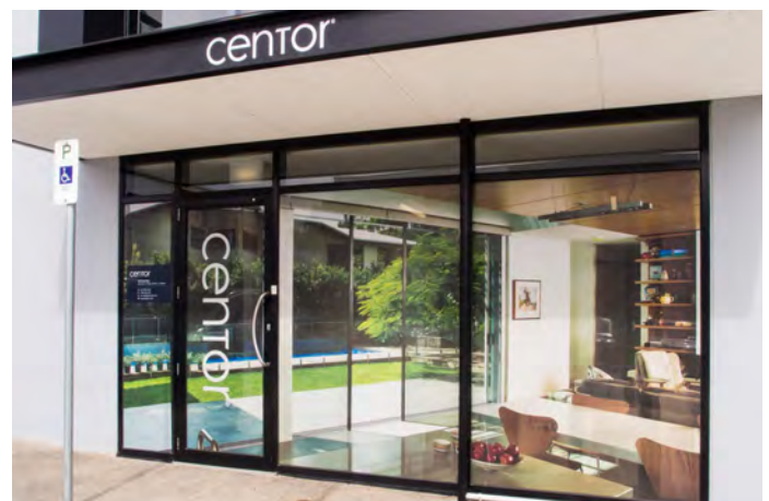
This is an example of a printed one way vision film. Note how the back layer is black to improve visibility from the inside out.
